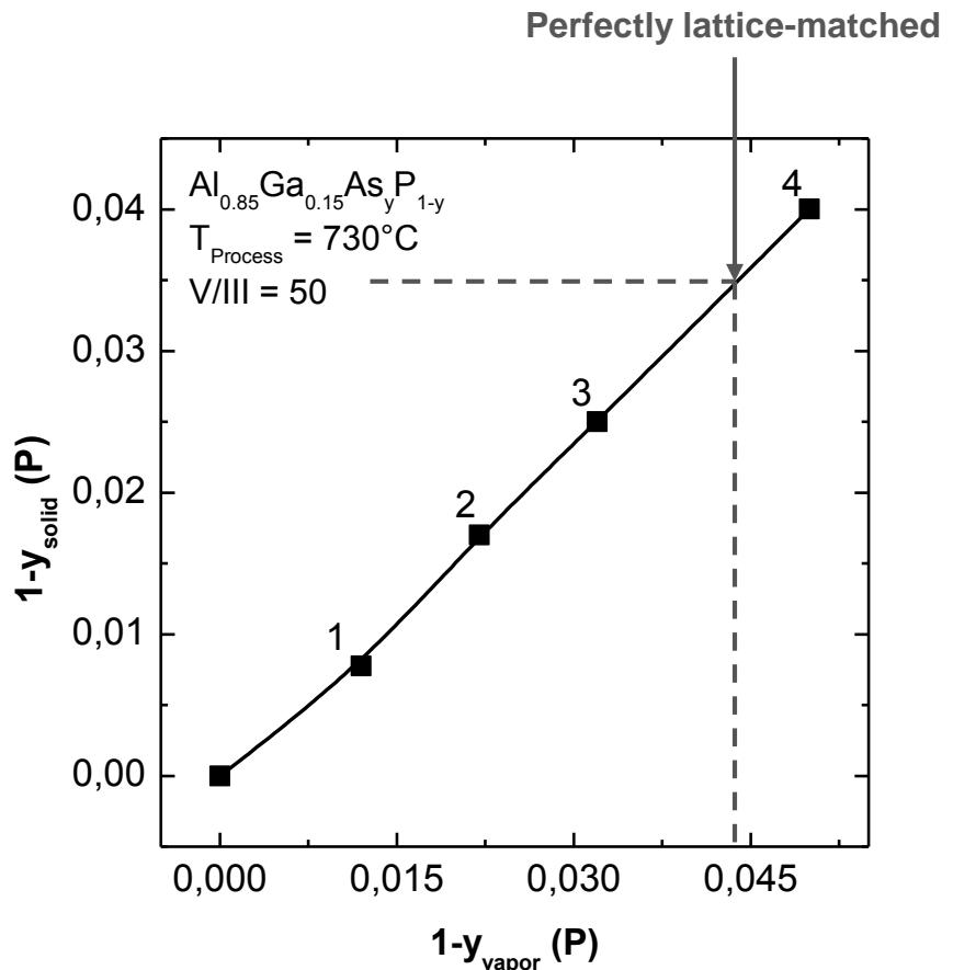
→ Adding ~3.5% of phosphorus to  $\text{Al}_{0.85}\text{GaAs}$  leads to exact lattice matching to  $\text{GaAs}$  at room temperature
