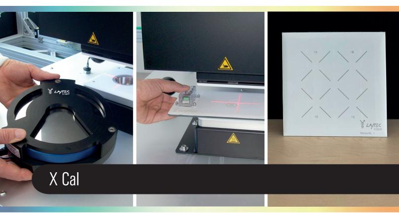
X Cal is a set of high precision equipment for on-site calibration of LayTec's X Link® systems. X Cal guarantees the high accuracy of X Link® systems, which is indispensable for process control and quality management in solar module production. It is recommended to calibrate X Link® after its delivery or moving as well as once a year to fulfill the requirements of quality auditors.
