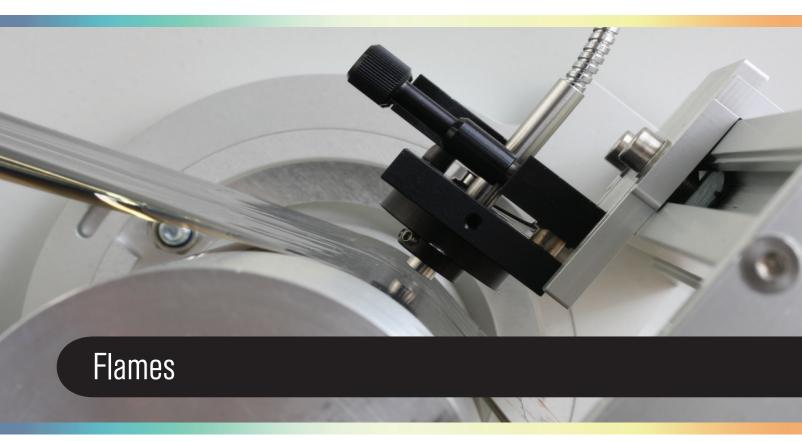
Flames IR is an in-line monitoring system for PV thin-film applications which monitors the key parameters of each layer during the process. It is available for CIGS and CdTe based thin-film solar cells and is compatible with typical in-line and roll-to-roll processes. Though the system is designed for thin film PV applications, it can be customized for many other large area coating processes on request.
