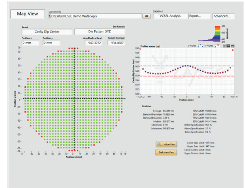
Fig. 1: Wafer-level 2D of cavity-dip center wavelength
