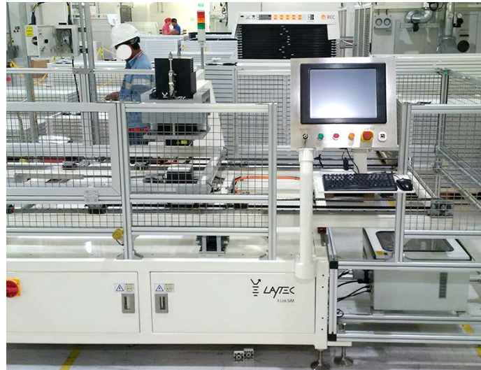
X Link® SAM – LayTec's mapping system for lamination control used in solar module production line at REC in Singapore
