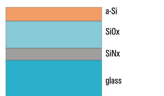
Fitting of optical model to in-line spectra gives thickness of all three layers.
