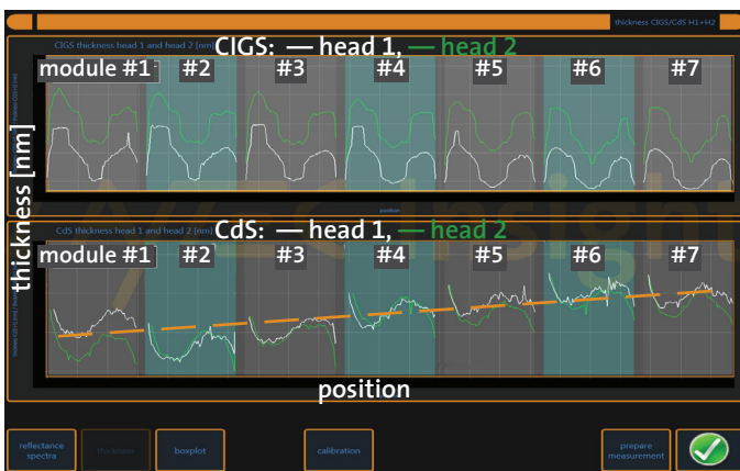
Fig. 1: Thickness transients of CIGS and CdS layers by SolR®.
