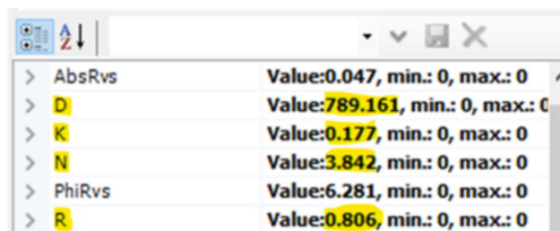
Fig. 2: Results window displaying the values for the thickness ( D ; in nm), the extinction coefficient ( K , dimensionless), the refractive index ( N , dimensionless) and the growth rate ( R ; in nm/s).
