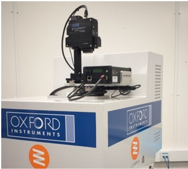
Fig. 3: LayTec's Etchpoint metrology system mounted on a PlasmaPro 100 Atomic Layer Etch system for endpoint detection.
