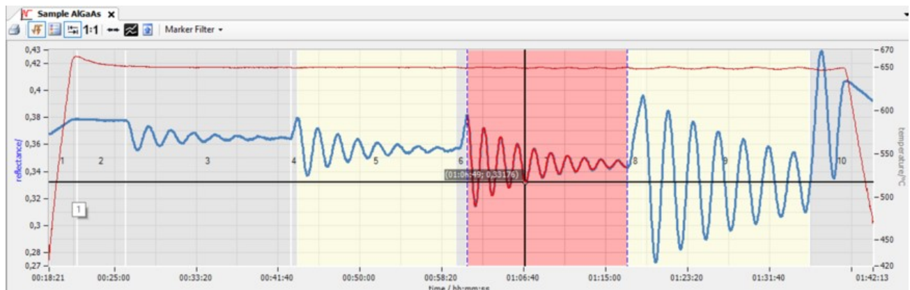
Fig. 1: Analysis screen of EpiNet® applying the 'NKR adv virtual layer fit' allowing for simultaneous fitting of the refractive index n , the extinction coefficient k and the growth rate r for analyzing materials like AlGaAs. Here, the fit was exclusively applied to the process step marked in red.
