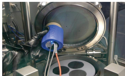
Fig. 1: AbsoluT attached to a shower-head reactor lid for calibration.
