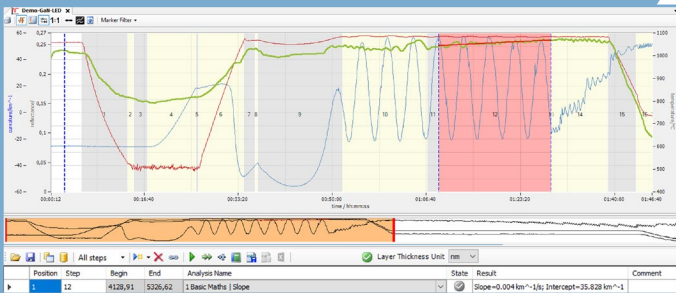
Fig. 1: Analysis screen of EpiNet® applying the “Slope” of the “Basic Math” package for deducing the gradient of the wafer curvature evolution from the curvature data line during the process step marked in red.
