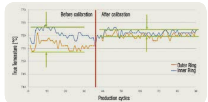
Temperature measurement with EpiTwin TT before and after calibration with AbsoluT
