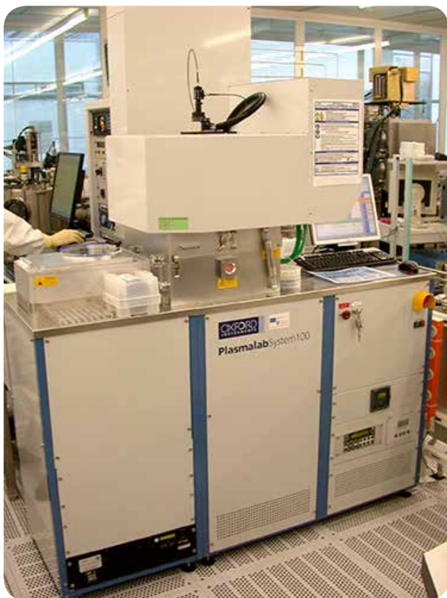
EpiTT UV installed on Oxford Instruments Plasmalab System 100 ICP CVD system to measure the layer thickness of \text{SiO}_2 and \text{Si}_3\text{N}_4 layers during deposition of a multilayer stack consisting of 50 alternating \text{SiO}_2 / \text{Si}_3\text{N}_4 layer pairs. By courtesy of Imenau Technical University.
