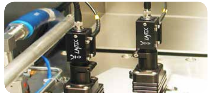
EpiTwin TT - the twin brother of EpiTT containing two measurement heads
