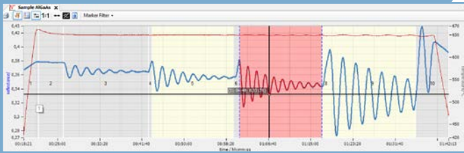
Fig. 1: Analysis screen of EpiNet® applying the "NKR adv virtual layer fit" allowing for simultaneous fitting of the refractive index n , the extinction coefficient k and the growth rate r for analyzing materials like AlGaAs. Here, the fit was exclusively applied to the process step marked in red.
