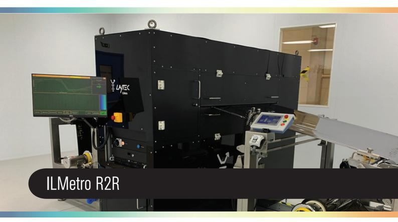
ILMetro R2R metrology stations combine several LayTec in-line metrology systems for a comprehensive control of industrial flexible thin film production processes by non-contacts measurements. If required, ILMetro R2R can drive the winder motors for transporting the substrate foil. Thus, complete mappings of roll pairs can be obtained in a fully automated mode. The measurement head compensates for residual waviness of the substrate foil for maximum robustness.
