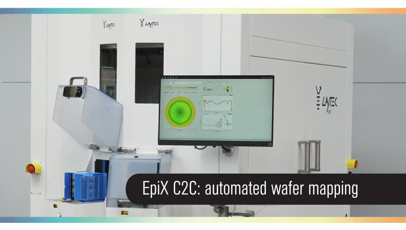
Combining white light reflectance and photoluminescence, the EpiX C2C system ensures a comprehensive 2D analysis of critical wafer properties by non-contact optical measurements. The cassette-to-cassette configuration of EpiX C2C allows to achieve the high throughput required in industrial applications.
