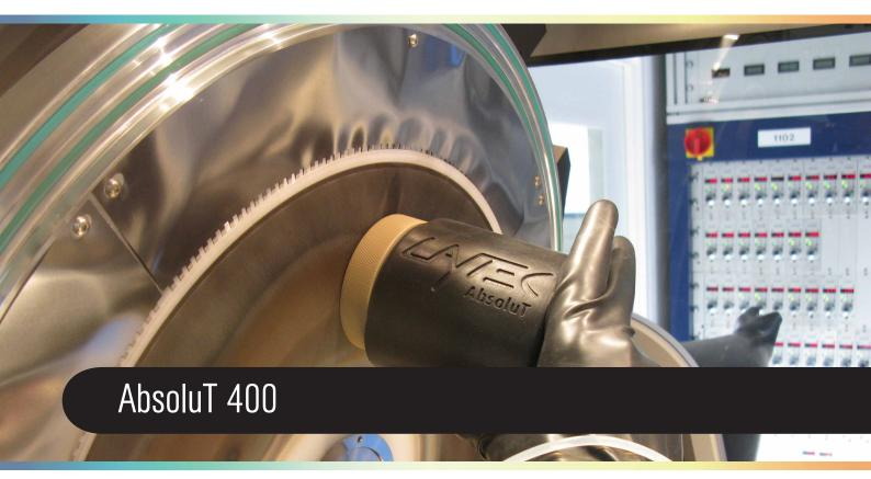
AbsoluT 400 is a high precision instrument for on-site temperature calibration of LayTec's Pyro 400 in-situ device on MOCVD reactors with an accessible viewport. It performs temperature calibration of Pyro 400 systems inside the MOCVD chamber through the original viewport. With AbsoluT 400 you can reduce the maintenance time and increase the reactor up-time.
