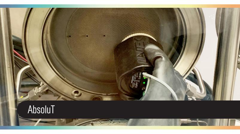
AbsoluT is a high precision instrument for on-site temperature calibration of LayTec's in-situ devices MOCVD reactors with accessible viewport. It performs temperature calibration of EpiTT and EpiCurve® TT systems inside the MOCVD chamber through the original viewport and alignment. With AbsoluT you can reduce the maintenance time and increase the reactor up-time
