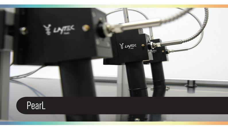
PearL is an optical in-line monitoring system, measuring photoluminescence spectra. The system is designed for measuring on CIS and CIGS based production lines. Photoluminescence spectra allow a fast detection of the effective Ga and Cu content of the absorber during the production process. A product option for CdTe absorbers is also available.
