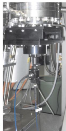
Fig. 1: Measurement setup installed at an oxide MBE chamber.
