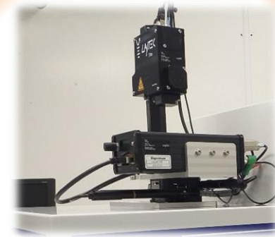
In-situ metrology during plasma etching
